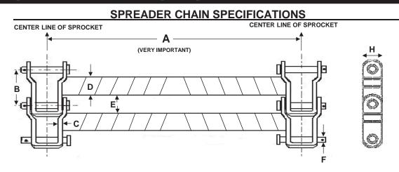
(A) SPROCKET - CENTER LINE TO CENTER LINE = \_\_\_\_ (IN INCHES)
